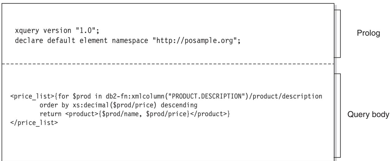
Figure 4. Structure of a typical query in XQuery
