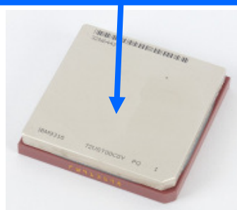
Single PU Chip without heatsink
