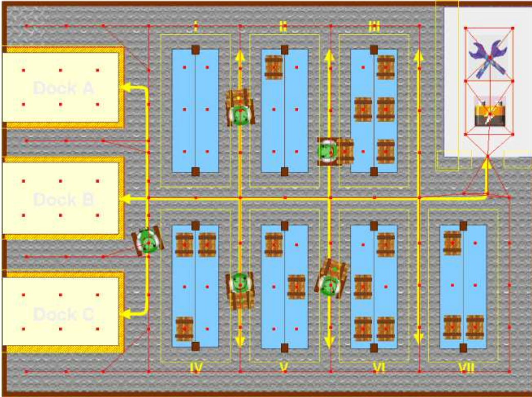
Figure 6.4: Storehouse floor plan overlaid with the way point reticle. The points and pathways are marked red (black). The obstacles are marked as yellow (white) rectangles.
